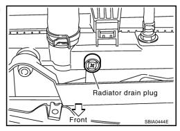
When draining all of engine coolant in the system, open water drain plugs on cylinder block. Refer to <a href="Mailto:EM-124">EM-124</a>, "DISASSEMBLY"</a>.
