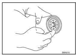
3. Screw oil filter manually until it touches the installation surface, then tighten it by 2/3 turn. Or tighten to specification.
